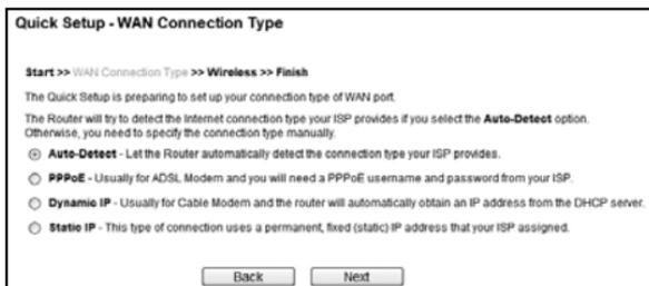
The Router provides **Auto-Detect** function and supports three popular ways **PPPoE**, **Dynamic IP** and **Static IP** to connect to the Internet. It's recommended that you make use of the **Auto-Detect** function. If you are sure of what kind of connection type your ISP provides, you can select the very type and click **Next** to go on configuring.
